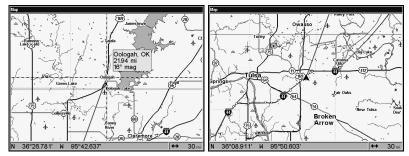
The 30-mile zoom figure (left) clearly shows the course line connecting your current position to your destination. The 30-mile zoom (right) shows current position and direction to destination on screen.
